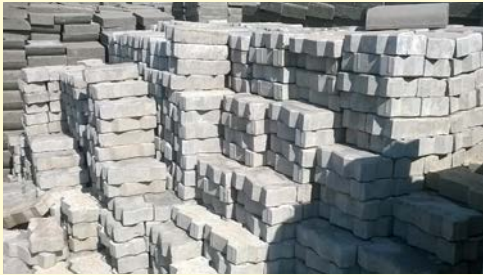
High-quality building material produced from processed C&D waste.
