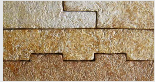
Detail of mycelium brick experiment, 2009. Ganoderma mycelium substrate.
